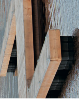
Coating comparison after 13 years outdoor exposure
